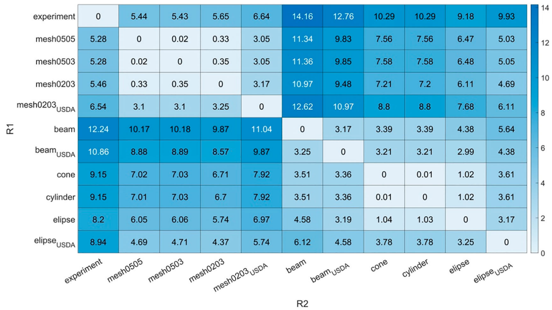
Figure 5. Matrix of average absolute relative differences between bending frequencies of all cases. The relative differences above matrix diagonal use the column (R1) cases as the references; the differences under diagonal use the row (R2) cases as the references.
