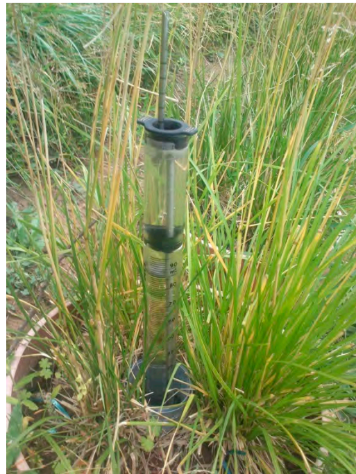
Figure A4. Measurement of cumulative water infiltration ( I ) in the non-rhizosphere soil zone of Deschampsia caespitosa L.
