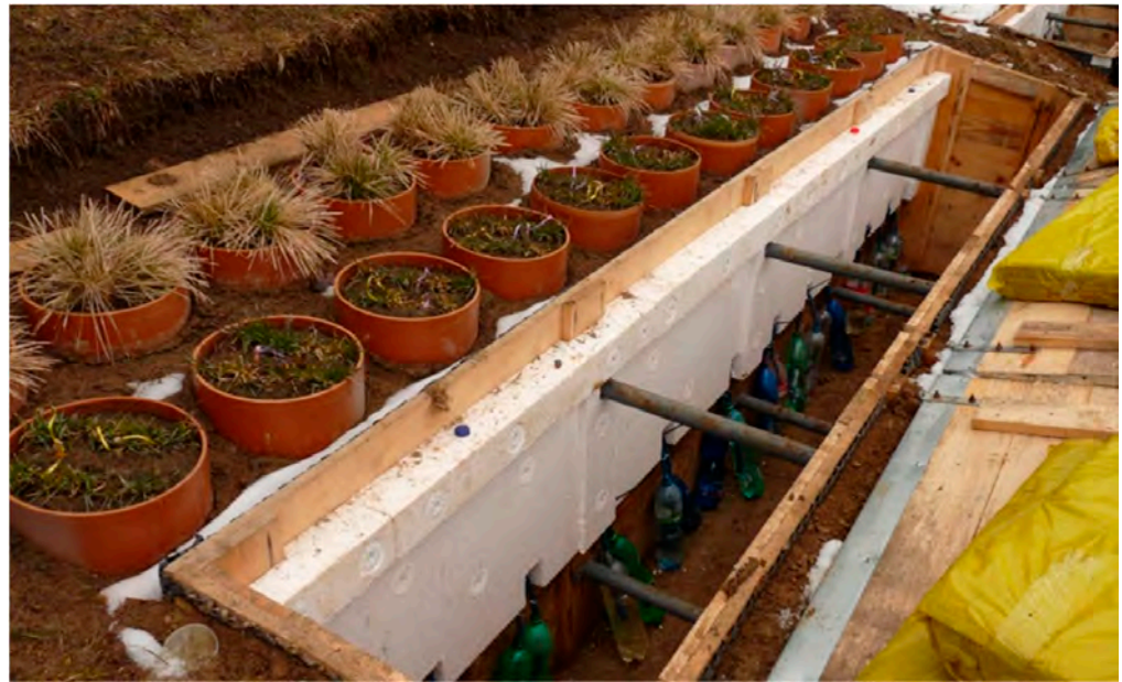
Figure A2. Control shaft with storage containers for catching the soil eluate.
