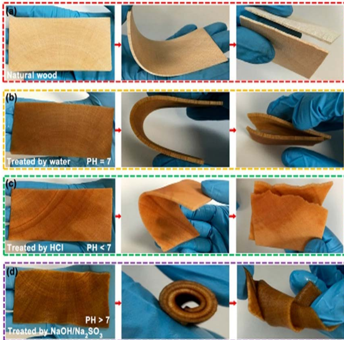
Figure 8: Some simple tests showing the final product flexibility after the treatment [114]. (a) Unmodified natural wood tissue, (b) water treatment done on natural wood tissue, (c) wood tissues are modified by HCl treatment, and (d) after NaOH/Na 2 SO 3 treatment, wood tissues become highly flexible.
