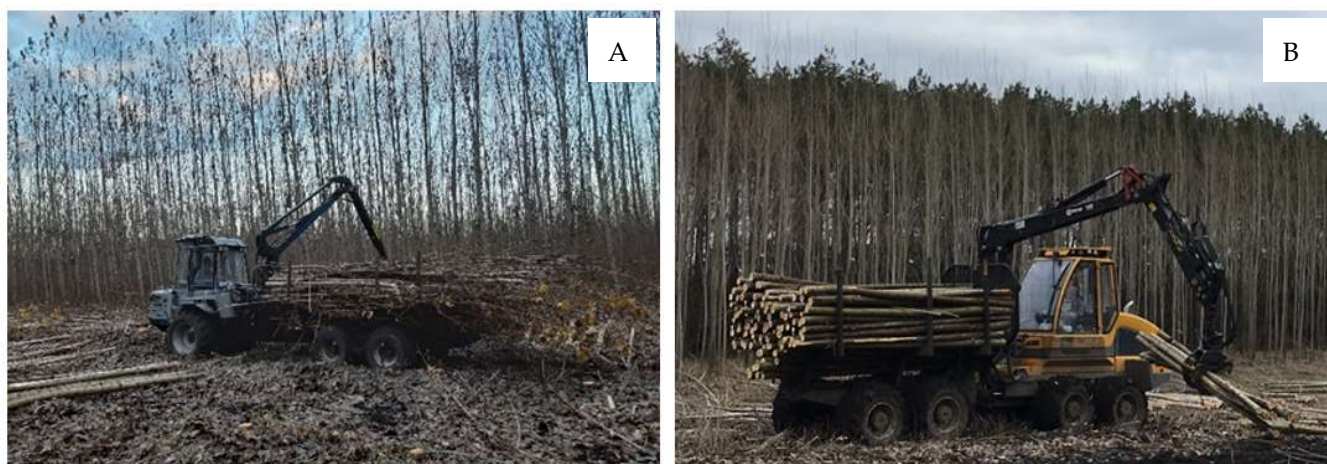
Figure 2. The two forwarders on the test: Vimek 610 (A) for the Vimek chain; Sampo FR28 (B) for all other chains.
