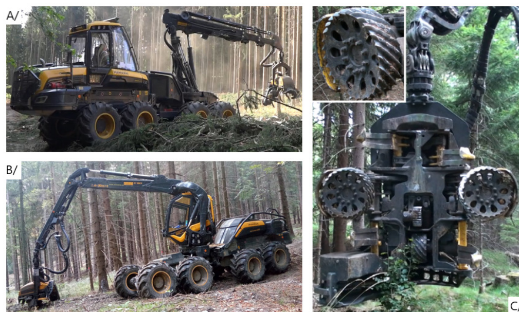
Figure 2. (A) Ponsse Ergo 8 W harvester; (B) Ponsse Scorpion King harvester; (C) Modifications of the H7 harvester head.
