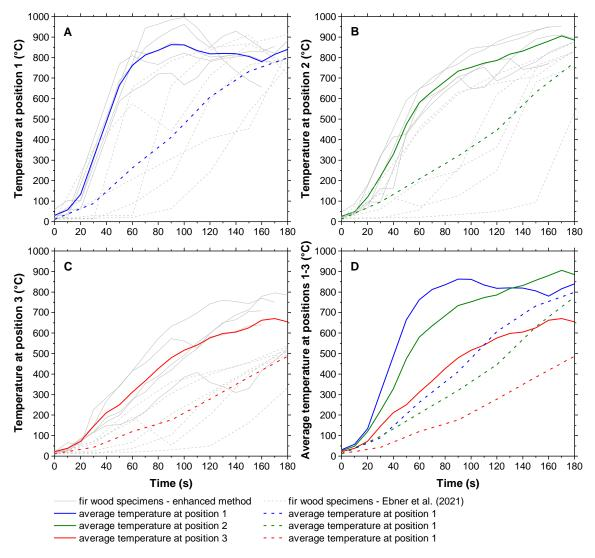
**Fig. 3.** Temperature-time diagram for the fir samples measured at positions 1, 2 and 3 (A through C) and the average temperature data (D). Solid line depicts values obtained by enhanced method, while dotted line stands for values recorded by Ebner *et al.* (2021).
