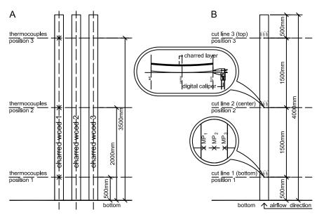
**Fig. 2.** Positions of the thermocouples at different heights in the wood chimney (A); and cut lines for the charred layer thickness (measurement points MP1, MP2, and MP3) and cupping measurements (B)
