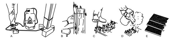
**Fig. 1.** The methodology of one-sided surface charring *via* the traditional Japanese yakisugi technique enhanced with propane gas ignition
