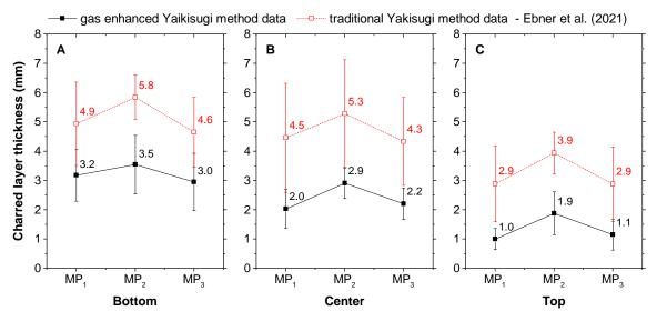
**Fig. 5.** The charred layer thickness at: cut line 1 – bottom (A); cut line 2 – middle (B); and cut line 3 - top (C) compared with previously measured data by Ebner *et al.* (2021) (Note: the error bars represent the standard deviation)
