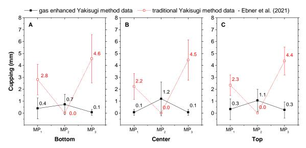
Fig. 6. The cupping at: cut line 1 – bottom (A); cut line 2 – middle (B); and cut line 3 - top (C)
