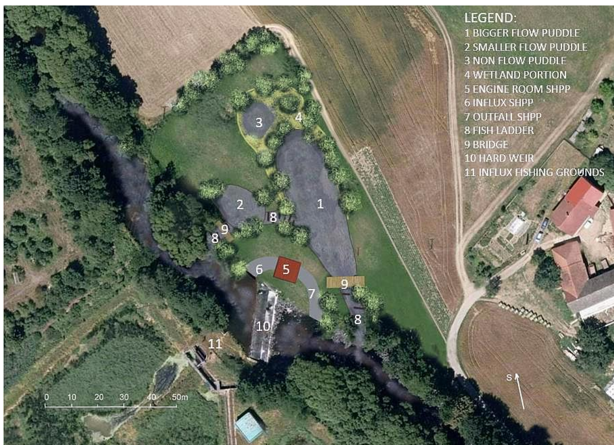
Fig 15. A schema of possible visualization of modification of left bank land (created by authors).
