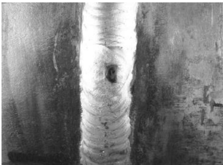
8: Deficiencies of surface and black spot sample 1 - JR3
