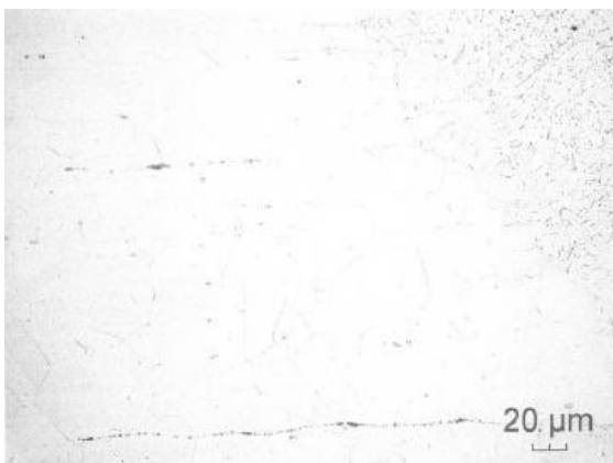
18: Sample 1-J3 400:1 Base material HAZ HNO 3 , HCl
