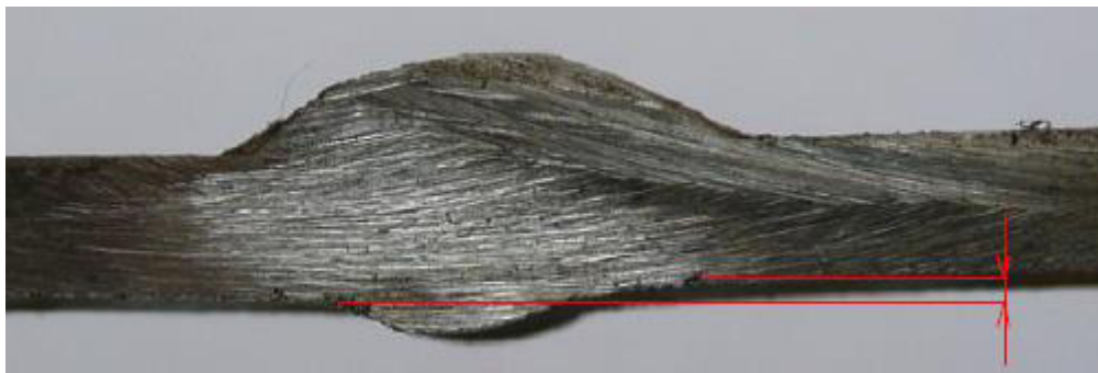
4: Detail Off-set root of weld
