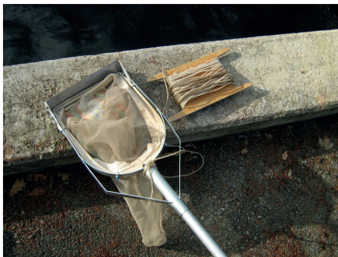
1: Adjusted sampling net with a cutting edge for taking samples from solid surfaces.
