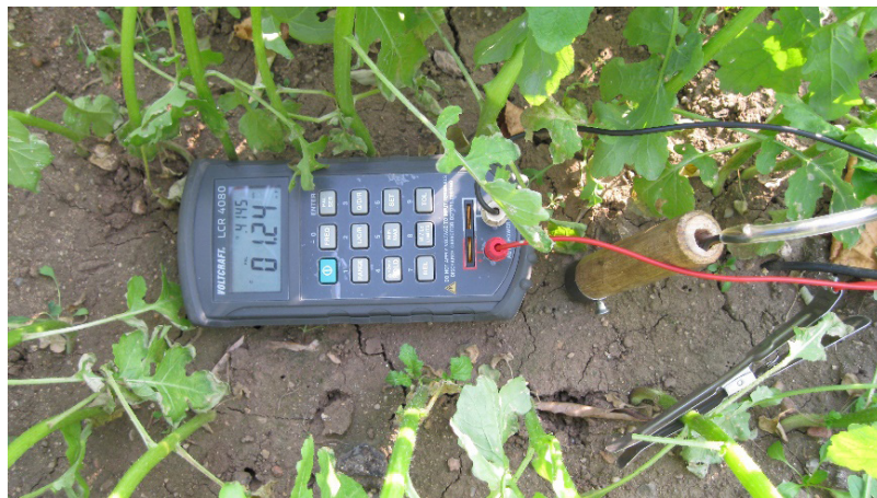
2: Non-destructive measurement of the root system of mustard plants in the stem elongation phase using an LCR device connected to two electrodes – needle (placed in the soil) and clamp (placed on plant base)
