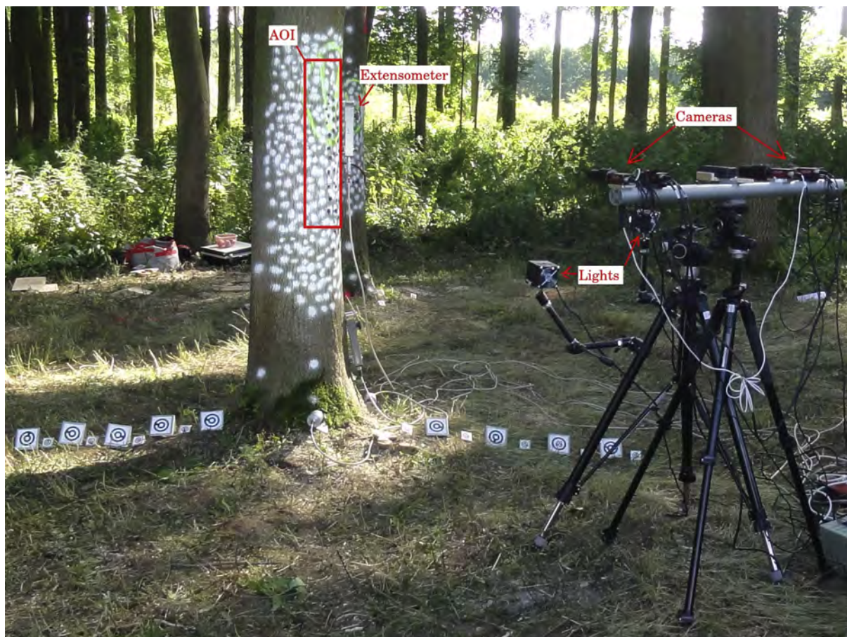
Fig. 1. Measurement setup at tree 1: stereoscopic video-camera set for image acquisition for subsequent 3D-DIC analysis.
