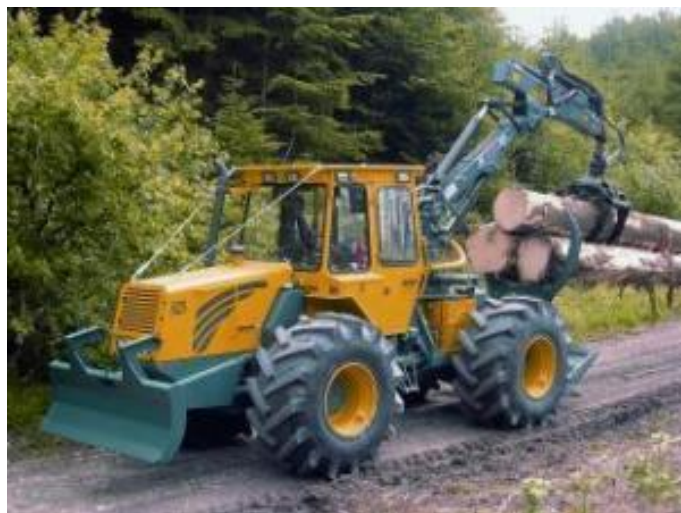
Fig. 101. Prime mover HSM 805 with the clam bunk, grapple on hydraulic boom and winch
