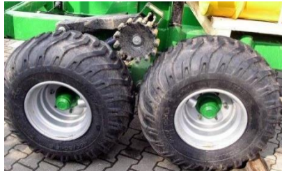
Fig. 104. Non-driven and pinion-driven bogie axle
