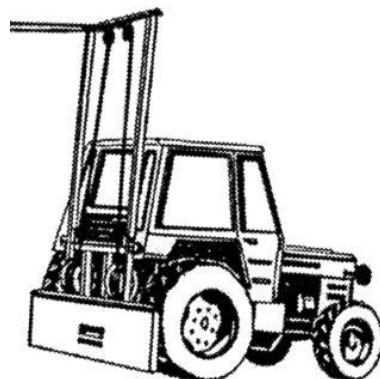
Fig. 73. Double-drum winch DTN-4 with turret
