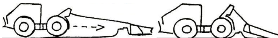
Fig. 88. Overcoming an obstacle by lifting the load
