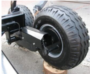
Fig. 104. Non-driven and pinion-driven bogie axle
