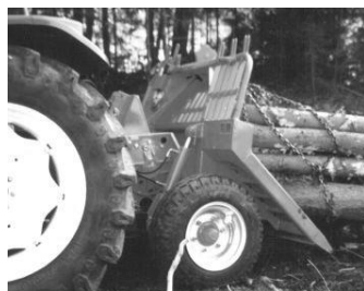
Fig. 76. Winch TIGER RW 80 with travel wheels
