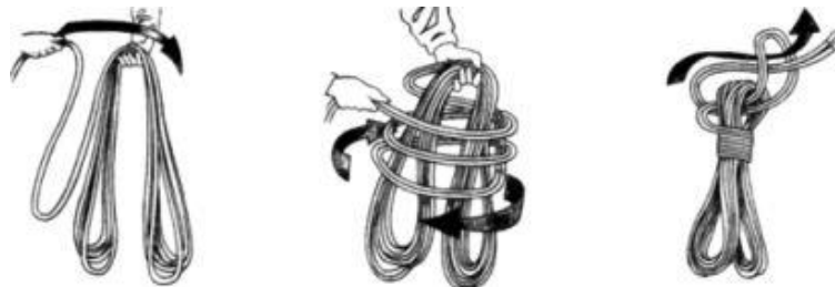
Fig. 73. Procedure of folding textile cables to scrolls
