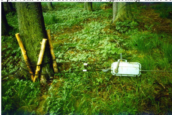
skyline tightening by manual winch
