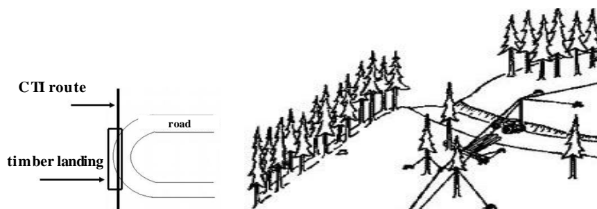
Fig. 81. Options of timber unloading under the skyline
