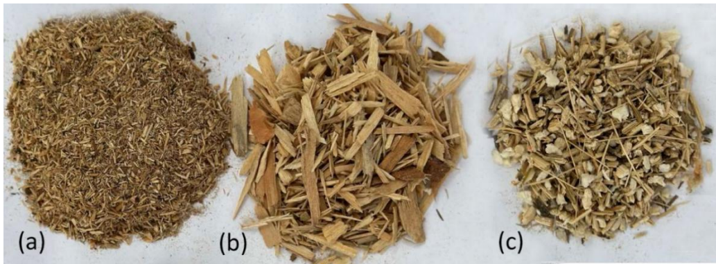
Fig. 2. Particles used in the manufacture of lightweight particleboards: (a) wood particles for the outer layers; (b) wood particles for the core layer; (c) sunflower stalk particles for the core layer.
