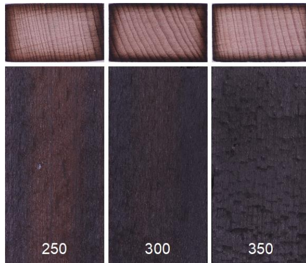
Fig. 7. The decay specimen surface (below) and charring depth (on top) after individual treatments; specimen cross section dimensions 15 \times 25 \text{ mm}^2
