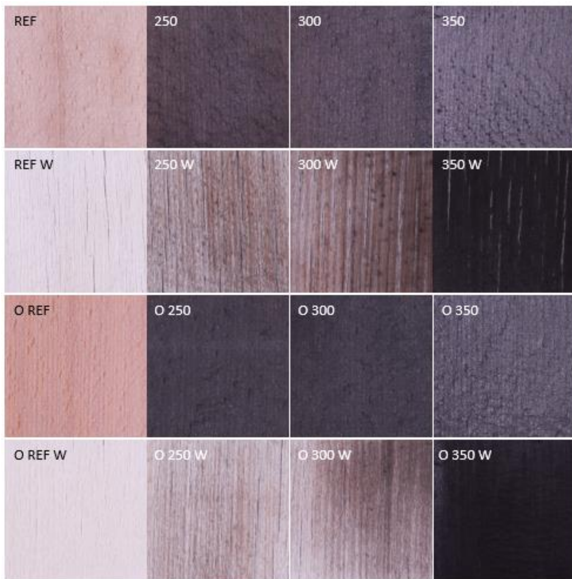
Fig. 1. Surface discoloration of artificial weathered specimens after 1000 h of exposure; REF – Reference; 250, 300, 350 – charred at different temperature; O – coated with linseed oil; W – artificial weathered
