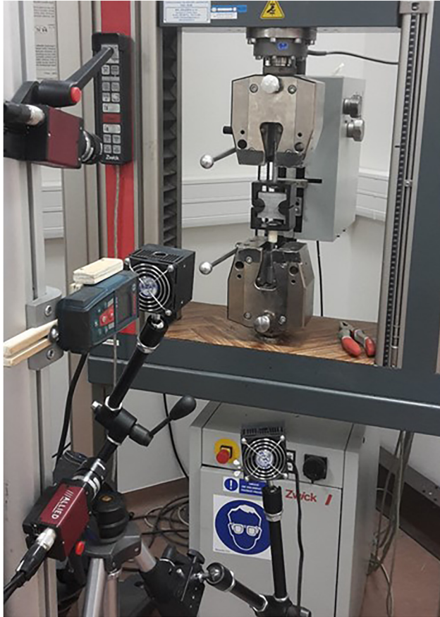
Figure 5: Experimental test configuration: stereo vision optical system (3D) of the tensile test perpendicular to the grain.
