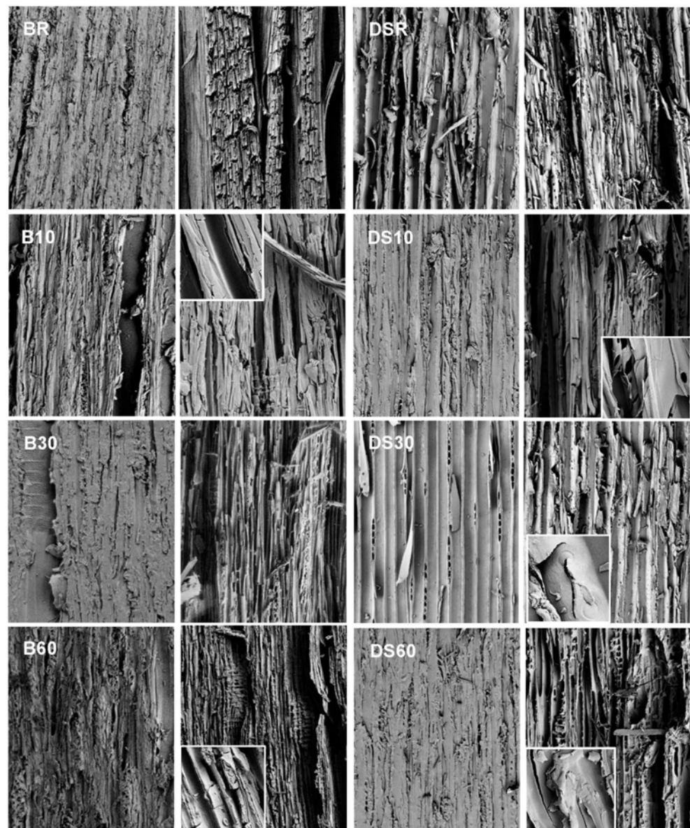
Figure 8. SEM images of birch (B) and dense spruce (DS) surfaces at a magnification of 100 \times . Left: inside stored references; right: artificially weathered specimens. Selected details in insets (at 1000–2900 \times magnification).
