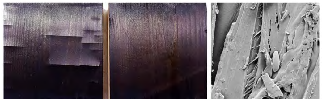
Figure 2. Samples DS60 with and without shallow surface checks pictured directly after modification. SEM image shows ruptured tracheid walls at 1000× magnification.
