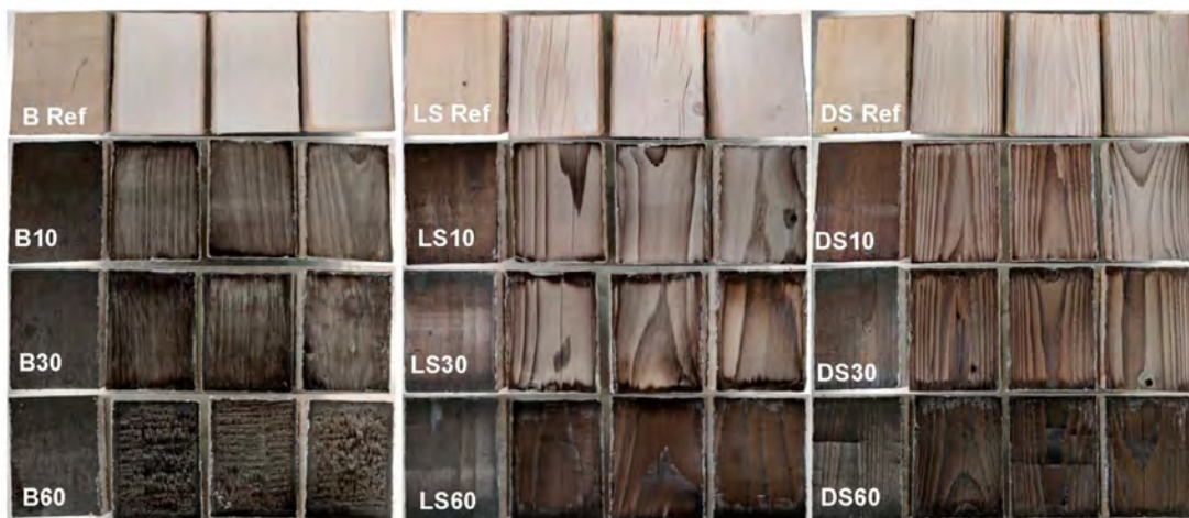
Figure 3. Weathered samples of birch (B), light spruce (LS), and dense spruce (DS) modified for different durations (10, 30 and 60 min) at 320 °C. The leftmost sample in the respected series is always the unweathered reference.
