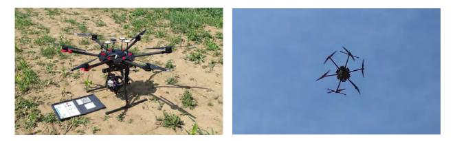
**Figure 3.** The six-rotor UAV DJI Matrice M600 with Micasense Altum camera on the ground with calibration panel (**left**) and during the flight (**right**).
