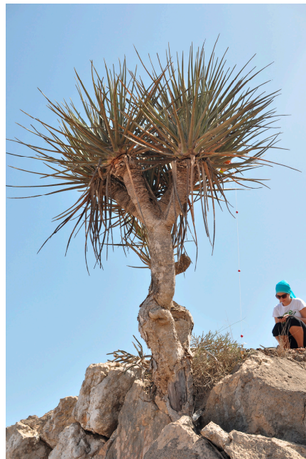
Figure 3. Prism points with a predefined distance in perpendicular vertical to the Earth's surface. Beads with a mutual distance of 50 cm suspended on a rope ending with the lead are used to define dimensions in the resulting 3D tree point cloud.
