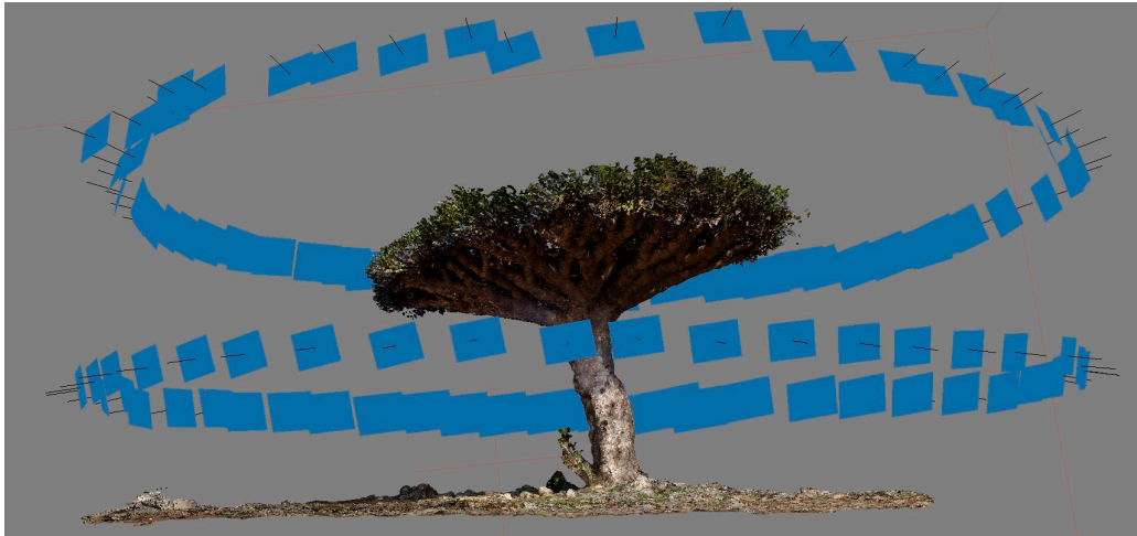
Figure 2. Method b)—position of captured photos to create a photogrammetric 3D tree point cloud. Two circles of photos capture the tree from two vertical angles. The upper circle captures the crown surface, the lower circle captures the stem and the inner structure of the crown.
