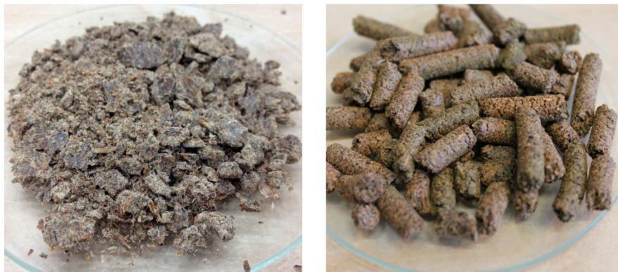
Figure 1. Seed cakes: (a) Milk thistle seed cakes are produced by seeds pressed through a hydraulic press; (b) hempseed cakes are formed by seeds extruded through a screw press.
