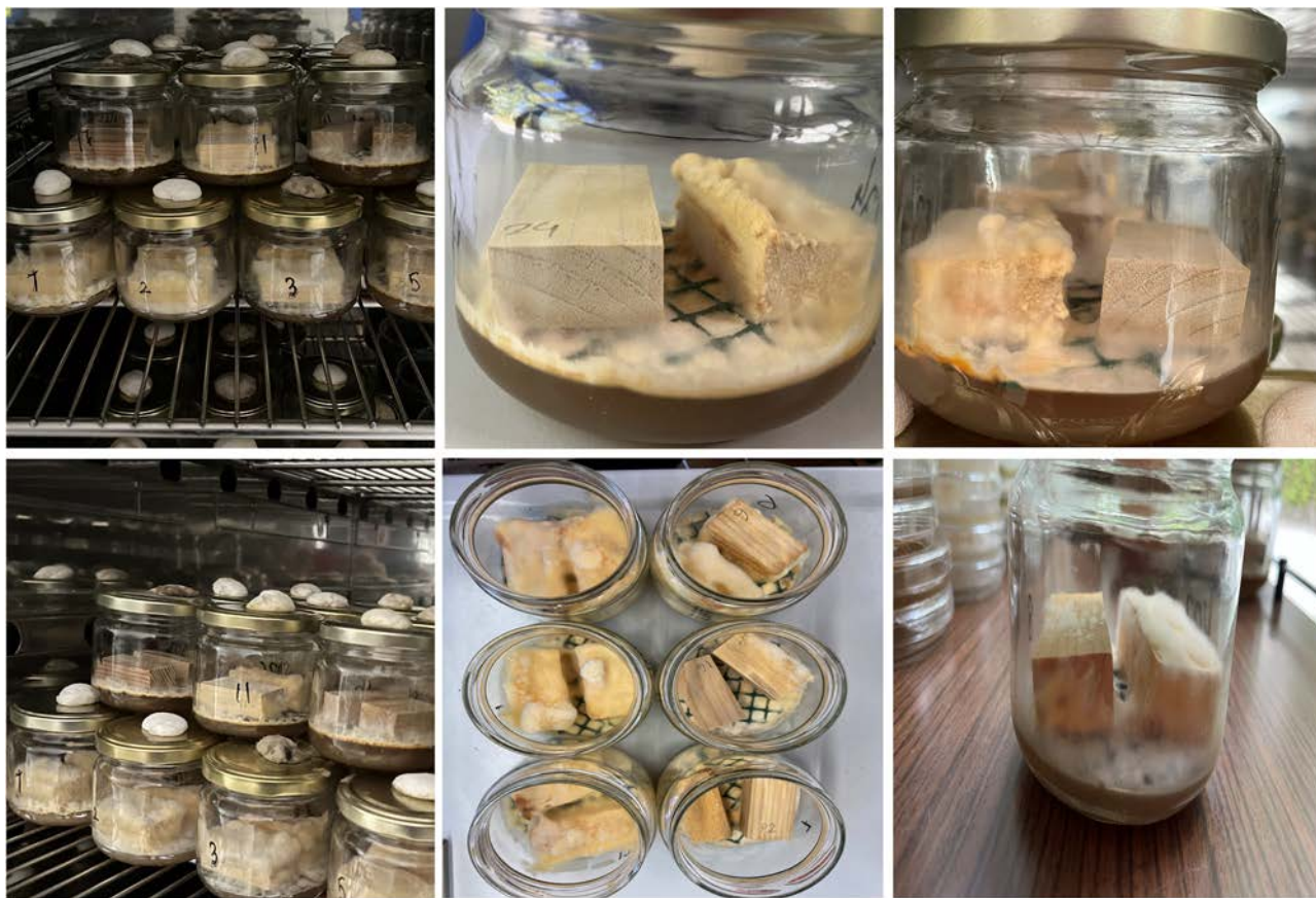
Figure 14: Fungi resistance experiment images of treated and untreated wood.
