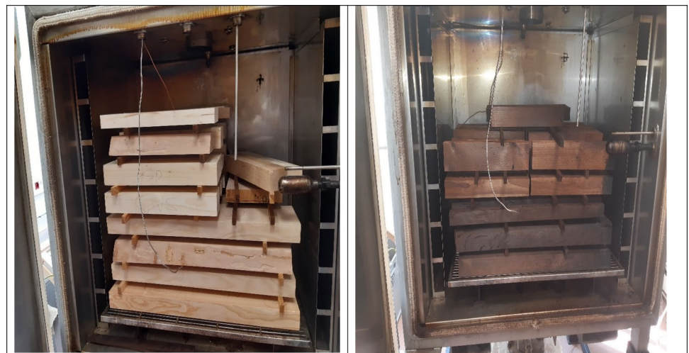
Fig. 1 The thermal modification chamber before and after the thermal modification
