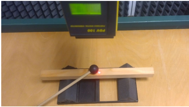
Fig. 2 Vibration sensing setup of a freely supported specimen, excited by a rubber hammer
