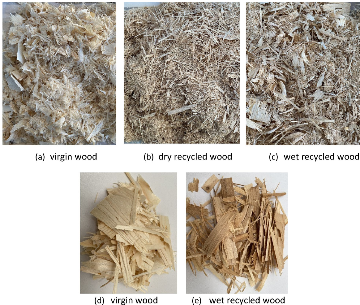
Fig. 1 Strands used for the manufacture of strand boards: a , b and c after disintegration; d and e after screening ( >10 mm)
