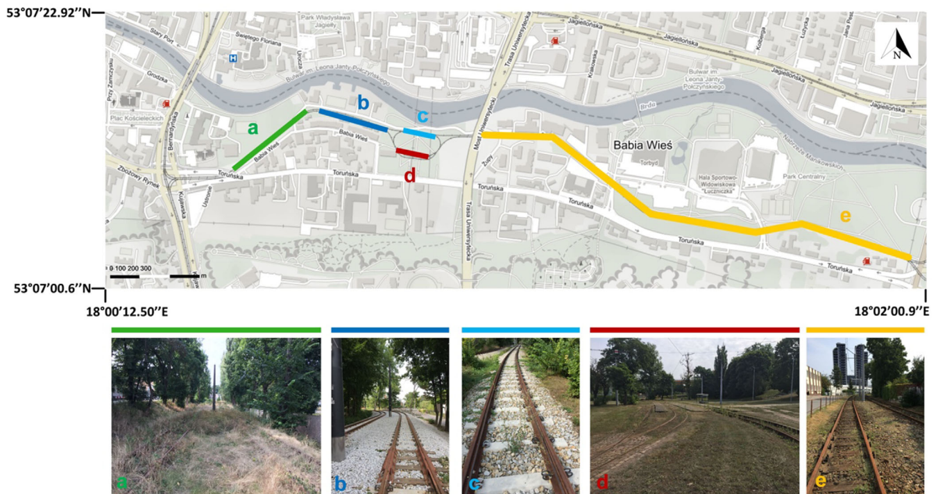
FIGURE 1 Demarcation of tram line and loop (a) unused and unused tram line section (Unused line); (b) newly reconstructed tram line section (New line); (c) newly reconstructed tram loop section (Loop rec); (d) old, maintained part of tram loop (Loop old); (e) unused and maintained tram line section (Old line). [Colour figure can be viewed at wileyonlinelibrary.com ]
