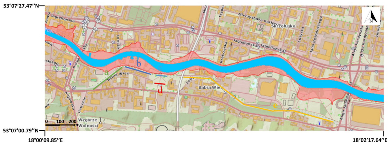
FIGURE 2 Map “Flood Risk Management Plan” in the study area (blue riverbed, red floodplain). [Colour figure can be viewed at wileyonlinelibrary.com ]
